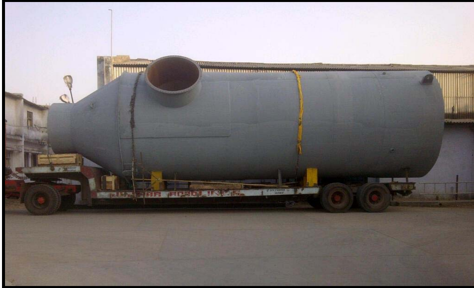
Water Seal Drum (3.8 m dia.) Ready for Dispatch from our works for OMPL Mangalore
